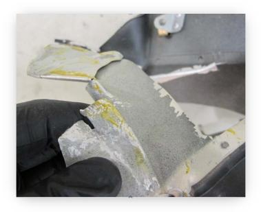
Figure 9: Yellow Paint Transfer on the Cockpit Structure
