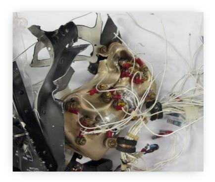
Figure 7: Dent in Right Side of Instrument Cluster
