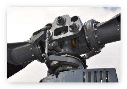
Figure 16: R44 Main Rotor Head (Source: https://commons.wikimedia.org/wiki/File:R44\_rotorhub.jpg)
