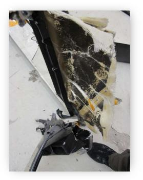
Figure 8: Yellow Paint Transfer on Cockpit Canopy Bow
